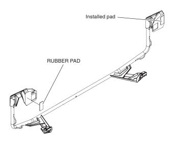
Install two Honda Pro-Connect<sup>TM</sup> latches into the rear carrier extender using a rubber spacer between each latch and the carrier extender. Secure the latches to the front carrier extender by installing a snap ring onto each latch from underneath the carrier extender.
