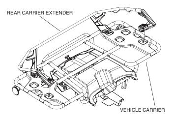
Secure the cargo box to the vehicle by pressing down each Honda Pro-Connect<sup>™</sup> lever.
