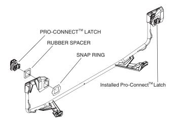
3. Lift the lever on each latch to unlock them. Place the rear carrier extender onto the rear carrier of the ATV. Line up each latch with its corresponding hole in the carrier then push each latch into its hole.
